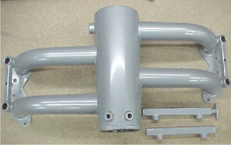
10/14/99 Intake manifold and fuel rails after powder coating
