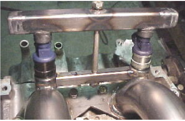
10/14/99 Intake manifold and fuel rails after powder coating
