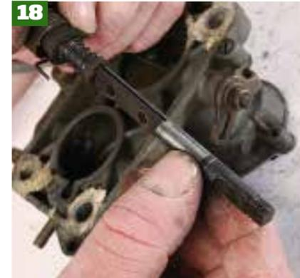
Then remove the throttle shaft from the main body and check for wear. Repeat steps 16 and 17 for the secondary shaft, remove and then check for wear. Finally remove the auxiliary venturis by hand or gently persuade with a pair of pliers.
