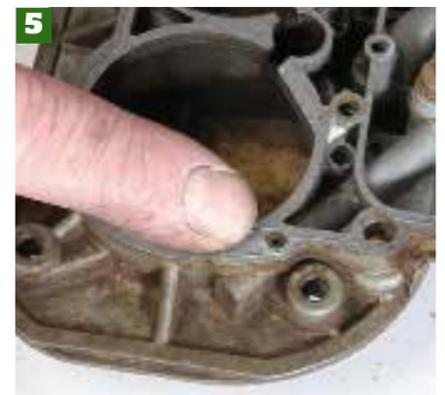
Test the power valve diaphragm by pushing down on the spring and blocking the small airway on the face surface. If the diaphragm is good the vacuum created will mean the spring will stay compressed, if it doesn't the power valve will need replacing.
