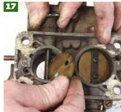
Undo the two screws that hold the butterfly in place and remove the butterfly. If they are tight gently tap with a hammer to loosen.
