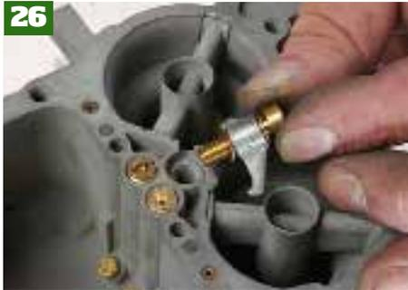
Refit the accelerator pump jet and delivery valve in the centre of the main body.
