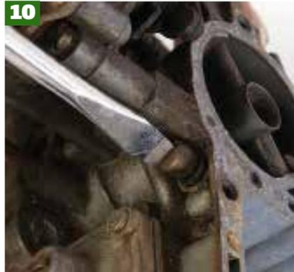
Remove the idle jet and progression jet from the sides of the float bowl.
