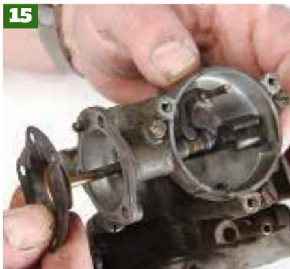
Then remove the three screws that hold the choke pull-off diaphragm in place and remove the diaphragm itself. Check it is in good condition, if not a replacement will be needed. Then remove the choke unit from the main body by undoing the three retaining screws at the side.
