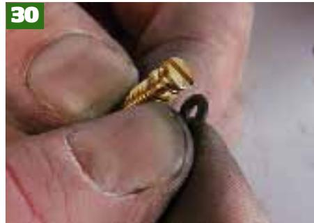
Next refit the mixture screw in the side of the main body, replacing the O-ring with a new item. To roughly get the right mixture wind the screw in all the way then unscrew by two turns.
