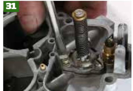
Refit the power valve diaphragm and float needle valve into the top of the carb then the filter with the new item from the service kit and replace 19mm filter nut. Once again new diaphragms are available.
