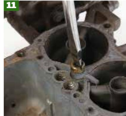
Now remove the accelerator pump jet and delivery valve from the centre of the main body.
