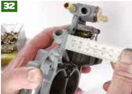
The next job is to refit and set-up the floats. Plastic floats need to be 35 mm from the surface and brass ones need to be set-up at 41 mm.
