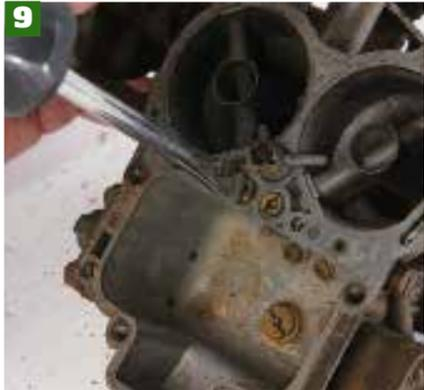
Remove the air corrector jets from the top surface and the main jets from the float bowl. Also remove the emulsifying tubes from under the air jets. It's worth writing down which size jets came from which place to ensure fitting them correctly later.
