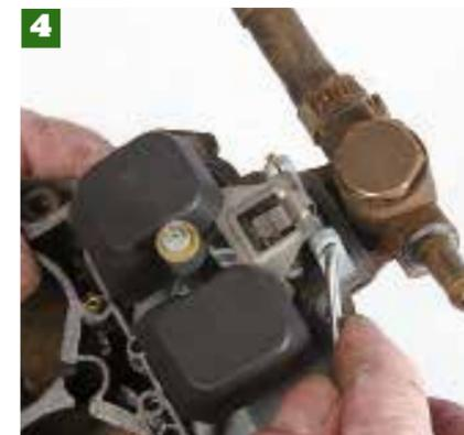
Remove the float pin with a small screwdriver, or if tight gently tap a small punch with a hammer. Then remove floats and float needle valve.
