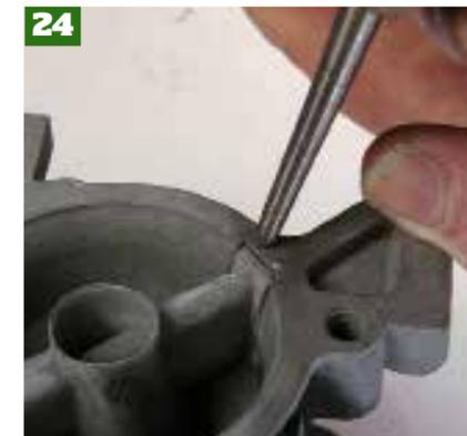
Next refit the auxiliary venturis. If they are loose they will rattle and will not work, so gentle tap the body with a hammer and punch to secure them in place.
