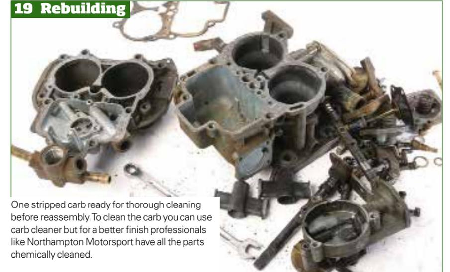
One stripped carb ready for thorough cleaning before reassembly. To clean the carb you can use carb cleaner but for a better finish professionals like Northampton Motorsport have all the parts chemically cleaned.
