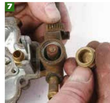
Then undo the 19 mm filter plug and remove the old filter. Remove the 10 mm float needle valve seat and the top half is ready for cleaning.
