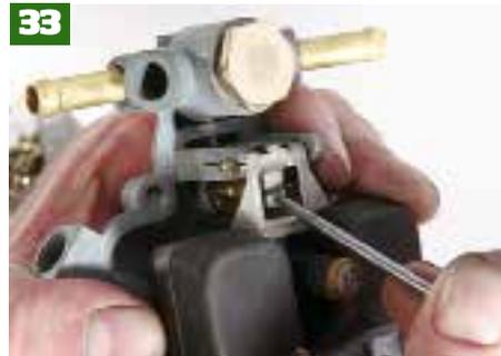
To adjust the distance between the float and the top of the carb gently push on the float tab with a screwdriver to bend it to the correct position
