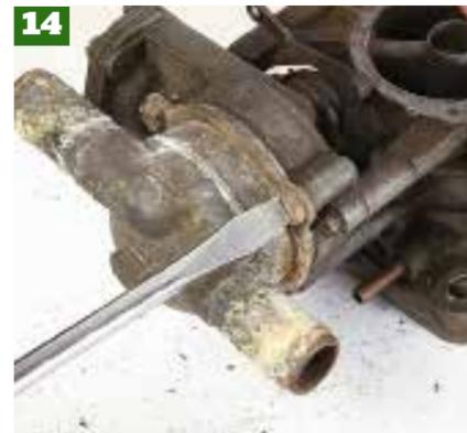
Remove the automatic choke housing (on the DGAV). If the unit works leave it alone as trying to repair them usually ends up with the centre bolt shearing off. If that happens the only way forward is to convert to manual choke as replacement auto choke parts are not available.
