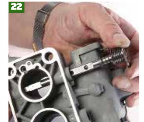
Now refit the throttle and secondary shafts into the main body. A drop of oil helps lubricate the shafts and makes life a little easier.
