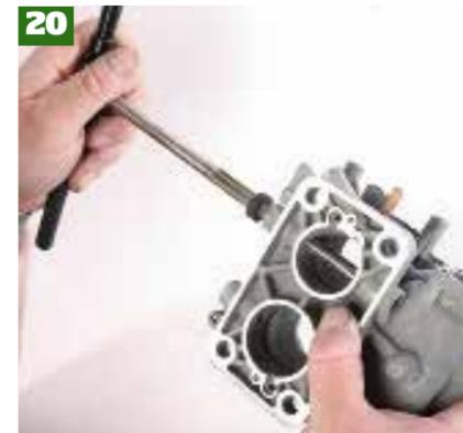
Before reassembling the carb Northampton Motorsport carry out a couple of trick mods. Firstly the base of the carb is machined totally flat to ensure a perfect seal with the spacer block. Also the body is reamed to accept Teflon bushes between the body and throttle shafts.
