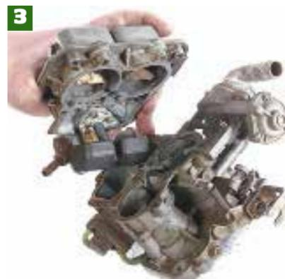
Then undo the six screws that hold the top on, and remove the top of the carb from the main body. Be careful as the screw heads are fairly soft metal.
