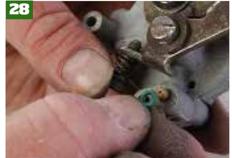
Refit the auto choke unit replacing the small green O-ring for the new one from the service kit...
