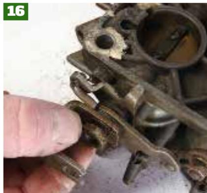
Turn the carb over to see the throttle butterflies. Remove the locking tab and 12 mm locking nut that holds the throttle shaft in position. Before removing the linkages and springs either write down or take a photograph of the order they come off in to help you remember how it all goes back together.
