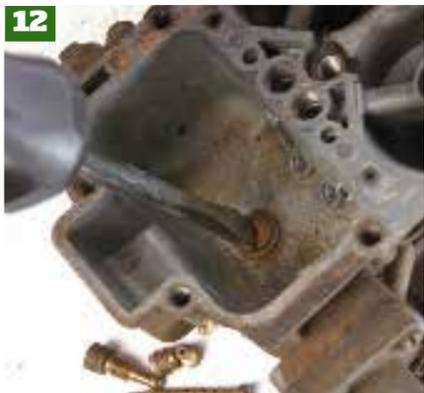
Remove the power valve from the float bowl.
