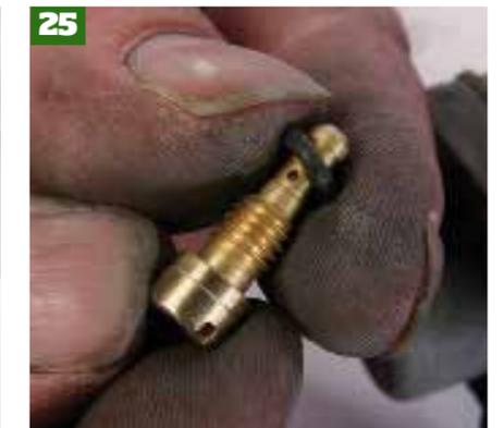
Before refitting the jets and emulsifying tubes replace the old O-rings with new ones from the service kit. Refit the jets in the same position you marked down earlier in step 9.
