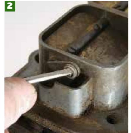
Now you can start stripping. Firstly remove the circlip for the choke butterflies with a small flathead screwdriver. Take care not to slip.
