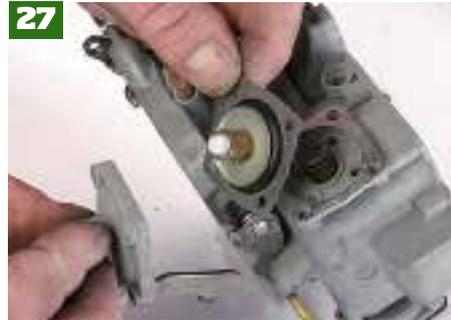
Next refit the enrichment device and accelerator pump, replacing both diaphragms with new items from the service kit.
