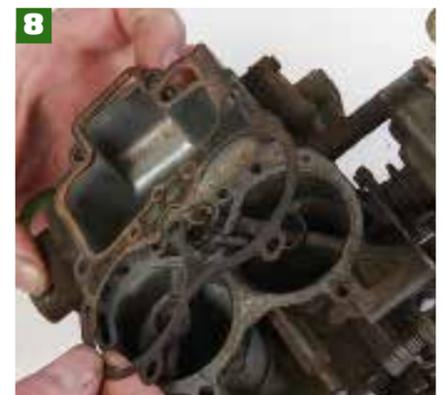
Now move on to stripping the main body of the carb. The first thing to go is the old gasket.
